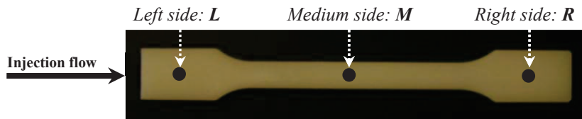
Figure IV-19: Tensile specimens' positions used for morphology observations in SEM.
