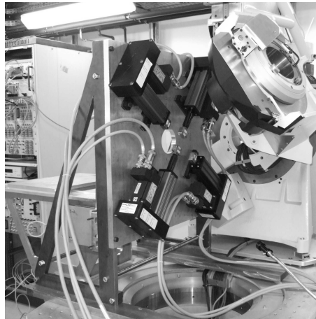
Figure 5.1: Multi-axial stretching machine in DiffAbs beamline in Soleil
