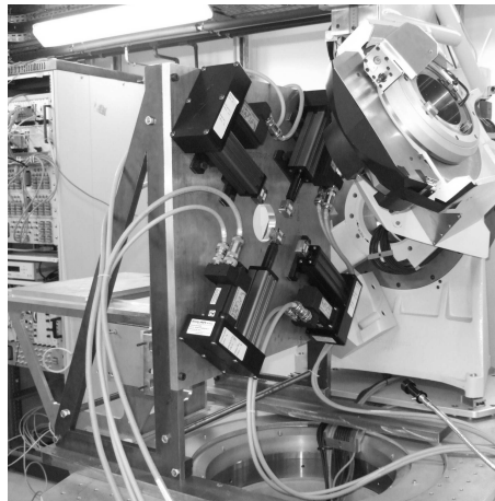
Figure 8.1: Uniaxial fatigue machine in DiffAbs beamline.
