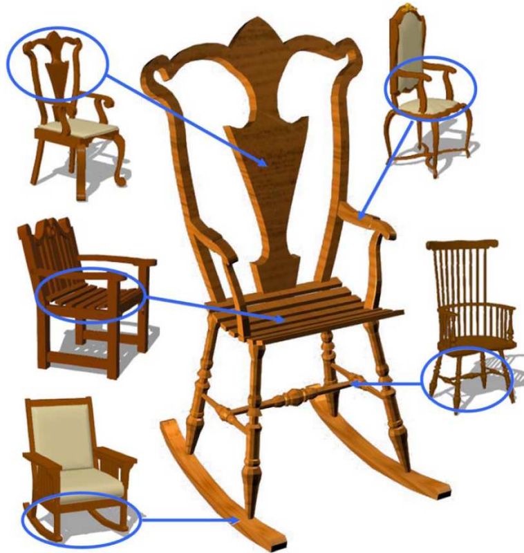
Figure 2.15 – Modeling a new chair composed from the circled parts of the others (FKS*04).
