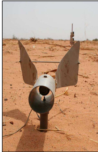
Figure 2.5 : salthophone installé sur PB (Photo : Abdourhamane Touré 2007)
