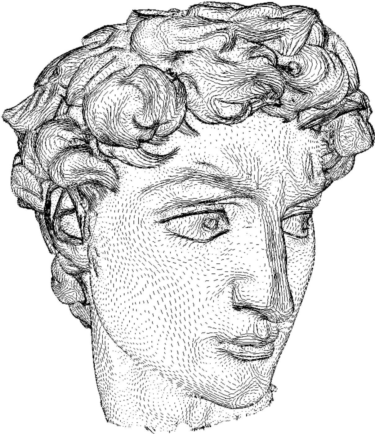
Figure 2.13: Directions of minimal curvature estimated on a mesh of Michelangelo's David. For each vertex, the averaging domain used for computations is the 2-ring of that vertex.
