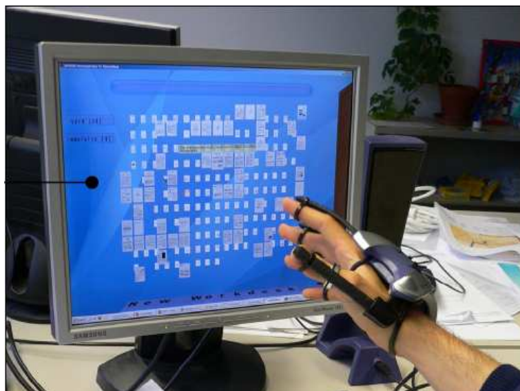
FIGURE 3.13: Illustration of a navigation technique based on the use of a data glove [17].
