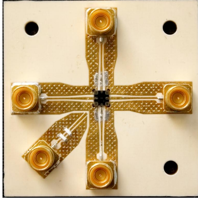
Figure 6.5: Photography of the RF chip-carrier with the sample inserted in its socket right in the center. The PCB is 4cm square, the sample 2.2mm large. The bonding pads of the sample can be seen in dark gold. They indicate the coplanar-waveguides ends on the sample, which dimensions match these of the CPW on the PCB. The electrical connection is done by aluminium wire bonding between the sample and the pcb. Via-holes of 200\mu\text{m} diameter are regularly drilled in the groundplane to ensure the potential continuity with the back ground plane.
