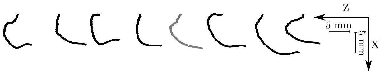
FIGURE 6.6 – Harpist forefinger movement during plucking actions. The grayed movement is used as reference for the robot.
