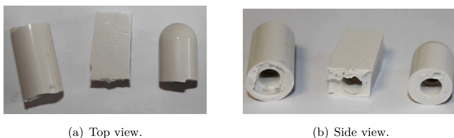
FIGURE 6.4 – Silicone fingertips of three different shapes : B-C-A
