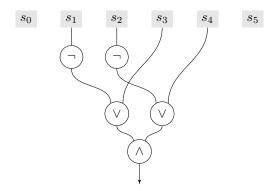
Figure 4.1: Example of a Boolean circuit defining a winning condition for the arena presented in Example 4. The winning condition defined is that if  $s_1$  appears infinitely often then  $s_3$  also appears infinitely often, and if  $s_2$  appears infinitely often then  $s_4$  also does.
