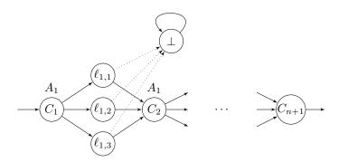
Figure 4.4: Module  $M(\phi)$ , where  $\phi = C_1 \wedge \cdots \wedge C_n$  and  $C_i = \ell_{i,1} \vee \ell_{i,2} \vee \ell_{i,3}$
