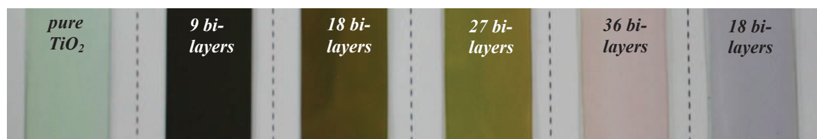
Fig.V-4: Photograph of the as-deposited films showing the range of colors produced for the different samples.
