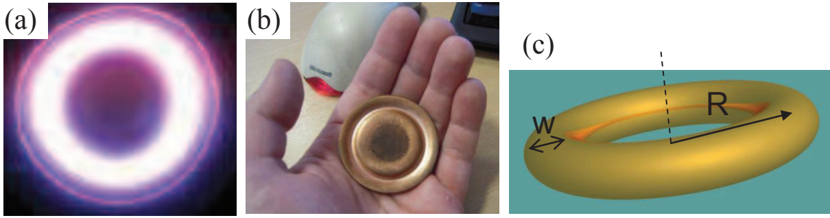
Fig.II-24: (a) Picture of an Argon plasma ring (Plasmionique), (b) Sputtering track on a Cu target, (c) Schematic of a torus.
