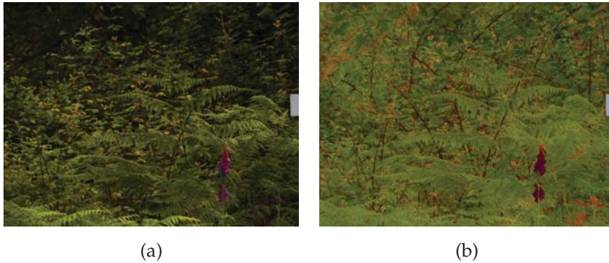
Figure 15: Example of true color composite of the (a) raw image, and (b) invariant representation by Ibrahim's method. The invariant composite clearly demonstrates how shadows and highlight have been removed so as to diminish the influence of the scene geometry. Nevertheless, it also decreases the meaningfulness of colors and shapes and makes the subjective interpretation more difficult.
