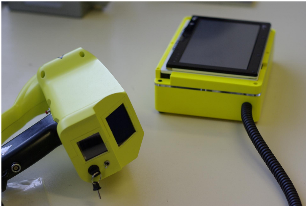
Figure 2.2: Portable LIBS device developed in Dijon's laboratory.
