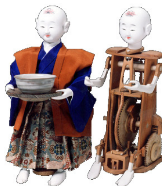
(b) Tea-serving karakuri ningyo and its mechanism. The automaton brings the tea cup while moving its feet as though it walked, although it actually rolls.
