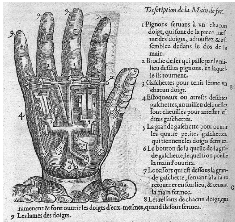
(a) The workings of a mechanical iron hand designed by Ambroise Paré (1585), and its descriptive text in Middle French. Because his education had been exclusively practical, Paré, who never attended medical school, knew neither Latin nor Greek, and was not accepted by his colleagues. He deliberately published his writings in French, against the opposition of the medical profession, but supported by the king and the intellectuals of his time. This was indeed an era of affirmation of French, and Paré clearly expressed in his works his desire “not to make the Arts cabbalistic”.
