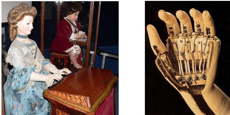
Figure 3.55 – La musicienne , made in the early 1770s by Swiss clock-maker Henri-Louis Jaquet-Droz (son of Pierre), and the mechanics concealed under its hands. The automaton comprises about two thousand and five hundred pieces.
