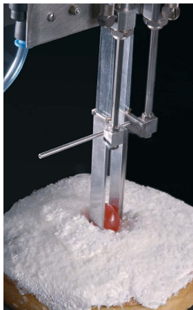
(c) Candied cherry gripper for the confectionery processing industry. Sticky workpieces cannot be accurately placed by conventional two-jaw grippers since they may remain stuck to their jaws. This gripper is made of two motionless jaws wrapped in a strip of moveable plastic tape.
