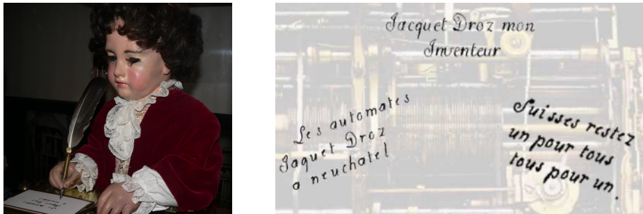
Figure 3.54 – L'écrivain , made in the early 1770s by Swiss clockmaker Pierre Jaquet-Droz, and examples of its writing. The automaton comprises about six thousand pieces.
