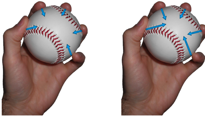
(b) Tightening forces. The sum of these contact forces is zero, so they do not produce any motion of the object, they are “pure” tightening forces. Obviously, the grasp on the right is more robust than the grasp on the left.
