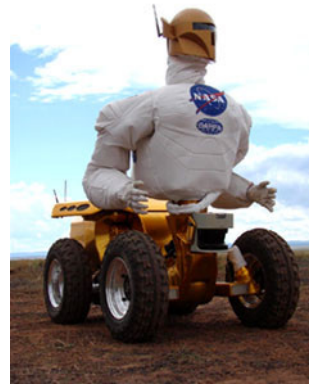
(b) A mobile exploration/manipulation robot made of a Centaur 1 four-wheeled rover and a Robonaut 1. It is shown here during a field test in the Arizona desert in 2006, near Meteor Crater.
