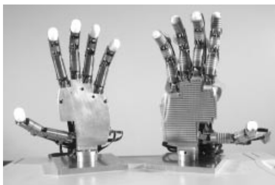
(a) The hand on the right is covered with the tactile sensor.
