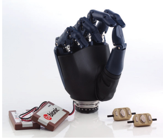
Figure 3.33 – RSL Steeper’s Bebionic hand, its batteries and its surface myoelectrodes. The protective cosmetic glove is absent.
