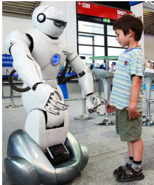
Figure 3.93 – Vietnamese robot Topio Dio at the robot fair where it was introduced (Munich, Germany, 2010). It is a small three-wheel humanoid, 125 cm, 45 kg, with five-fingered hands. It is envisioned as a service robot acting as waiter or bartender (Tosy Robotics 2011). Little information is available at the moment.
