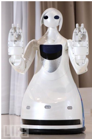
(c) Wheeled robot TPR-Robina, made by Japanese firm Toyota and used since 2007 as a tour guide at the Toyota Kaikan Exhibition Hall in Toyota, Japan (Toyota 2007). The robot is 120 cm tall and weights 60 kg. Its hands are three-fingered articulated grippers, designed to grasp pens to sign its name.
