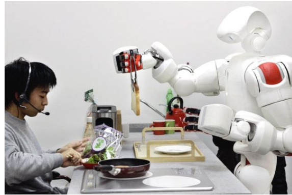
(b) The robot picks up a toast from a toaster and places it on a plate (prismatic precision grasp of the tongs) while a student prepares a salad, during a demonstration at Waseda University in 2007.
