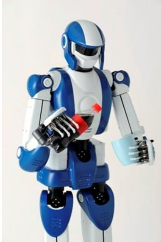
(a) HRP-4 pretending to serve coke. This humanoid robot by Japan's National Institute of Advanced Industrial Science and Technology (AIST) and Japanese firm Kawada Industries is the latest installment in their HRP series (AIST 2010; Kawada Industries 2010). Design was simplified and optimized, so that the robot is lighter and less expensive (151 cm, 39 kg, around $ 300 000). Despite having five fingers, the hands are limited to simple movements, since each hand has two degrees of freedom and a maximal payload of 0.5 kg.
