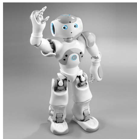
(d) The latest version of the entertainment robot Nao, by French company Aldebaran Robotics (58 cm, 5 kg, about 12 000 euros). Its three-fingered hands are articulated open/close grippers (Aldebaran Robotics 2011). They can seize and lift small objects, with a maximal payload of 0.3 kg using both hands.
