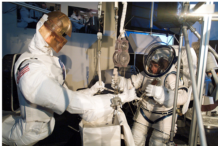
(c) A teleoperated Robonaut 1 participates in a test with an astronaut at NASA Johnson Space Center in 2003, to evaluate human/robot collaborative work. They are assembling an aluminium truss structure.
