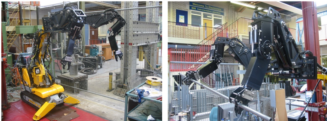
(a) This machine consists of a small vehicle with a hydraulic manipulator moving two seven-function manipulators (six rotational joints and a gripper).
