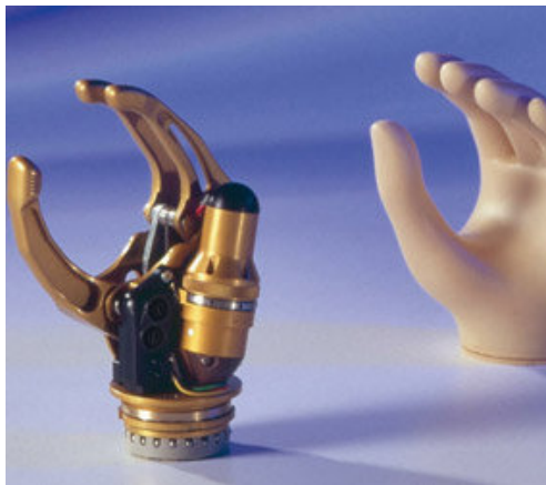
Figure 3.26 – A typical myoelectric hand: Otto Bock’s System Electric Hand, size 7, for teenagers and adults with small hands (Otto Bock 2010). It is an open/close three-jaw gripper in a PVC cosmesis.
