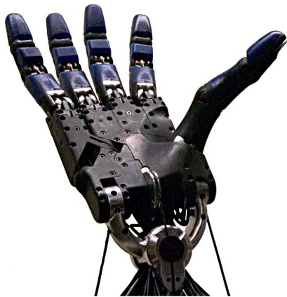
For compliant grasping, polyurethane pads are installed on the fingers (blue).
