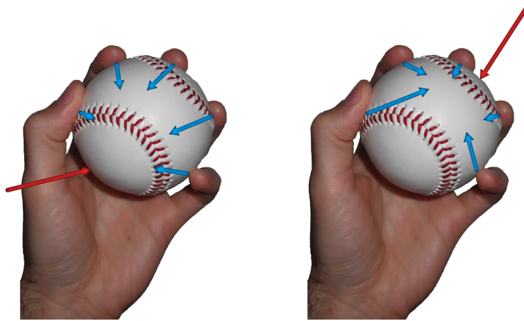
(a) Opposing forces. They cancel the external load in red (possibly a disturbance).
