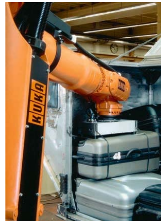
(d) Baggage gripper at the end of a serial manipulator, for use in airports. A machine braces both the baggage and the gripper with two plastic ties. The robot places the baggage in the air-cargo container, cuts the ties with an inbuilt knife, and throws them out for disposal or recycling. This design copes with any size, shape or weight, and places the baggage in nearly any position.
