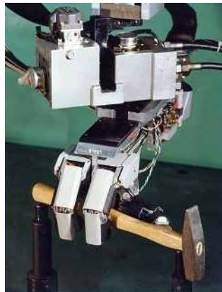
Figure 3.10 – UB Hand I, a three-fingered hand developed in the late 1980s at the University of Bologna, Italy
