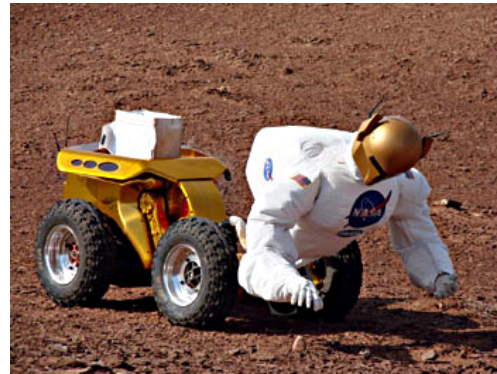
(b) Robonaut 1 mounted on a Centaur 1 four-wheeled rover, picking up a rock sample during a field test in the Arizona desert in 2006, near Meteor Crater. Such a mobile manipulation system is a good candidate for future exploration missions on Mars and the Moon.
