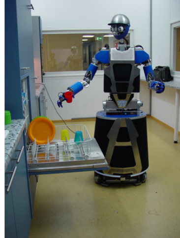
(b) Wheeled robot Armar III in the mock-up kitchen of the University of Karlsruhe, Germany (Asfour, Regenstein, Azad, Schröder, Bierbaum, Vahrenkamp, and Dillmann 2006). Its hands have five fingers and eight independent degrees of freedom each. The Armar robots are capable of artificial learning by interaction with the environment, meaning that they learn about objects by using them.
