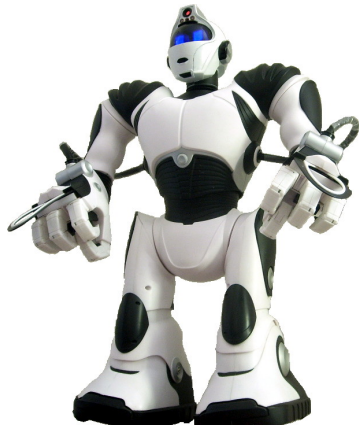
(a) The toy robot RoboSapien v2 and its oversized four-fingered articulated hands. Released in 2005, it is 56 cm tall and weights 3.6 kg (WowWee 2011).
