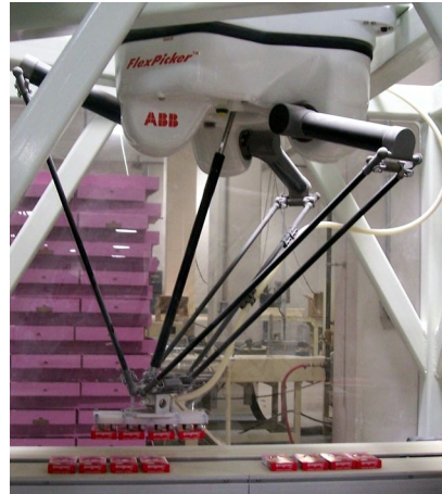
(b) Fast parallel manipulator with a four-at-a-time vacuum-based end effector. The white hose is the vacuum line.
