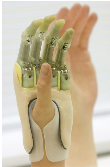
Figure 3.32 – Four ProDigits arranged into a myoelectric prosthesis for a transmetacarpal amputee
