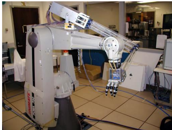
Figure 3.67 – A Utah/MIT Hand mounted on a Puma manipulator arm (1990s). The actuator package is fixed on the forearm of the manipulator; another possibility is to place it on an external mounting.
