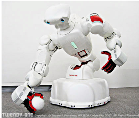
(a) The robot picks up an object fallen on the floor (spherical power grasp).
