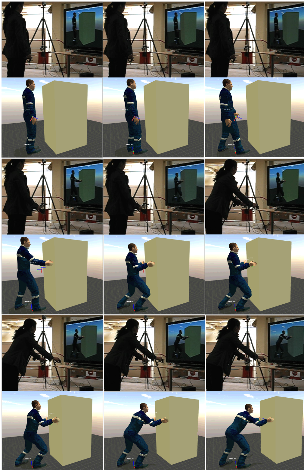
Figure 5.11: The virtual character pushing a storage cabinet through interactions with an operator.
