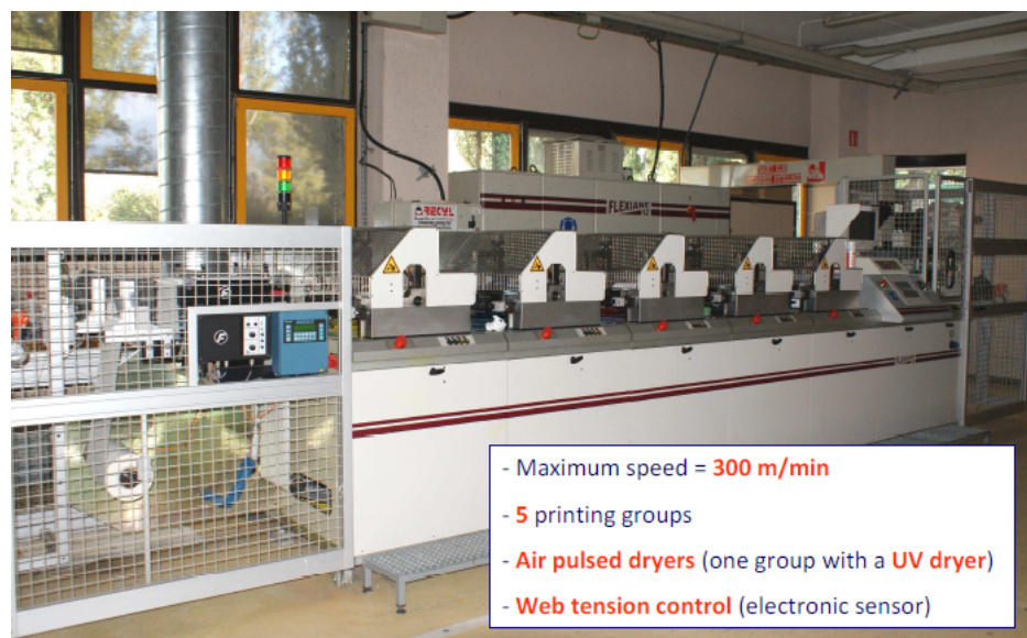
Figure 7.14: The Flexiane printing press and characteristics - Flexography pilot adapted to roll to roll printing
