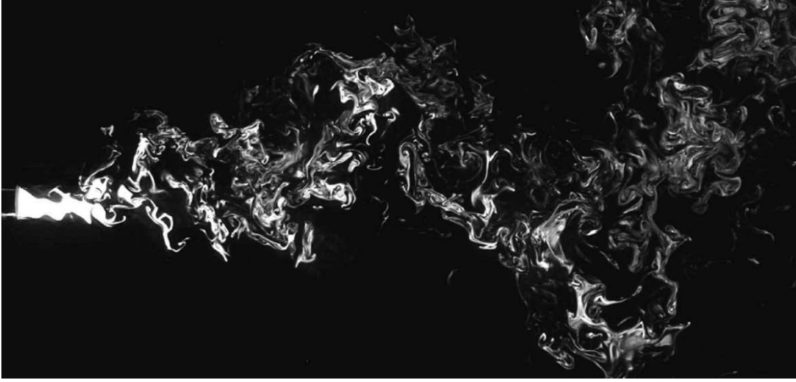
Figure 5.2: 2d image of a 3d turbulent flow: measurements of a fluorescent field done by shining a plane with an argon laser sheet through the water tank in a plane containing the axis of the mean flow. Image taken from Duplat et al. [2010b].
