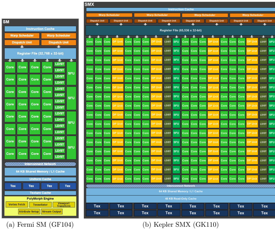
FIGURE I.12: Fermi vs. Kepler : architecture d'un Streaming Multiprocessor (© NVIDIA)
