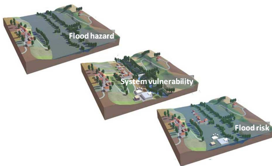
Figure 1.1. Flood risk as the conjunction of hazard and vulnerability. Source: prim.net 5 .
