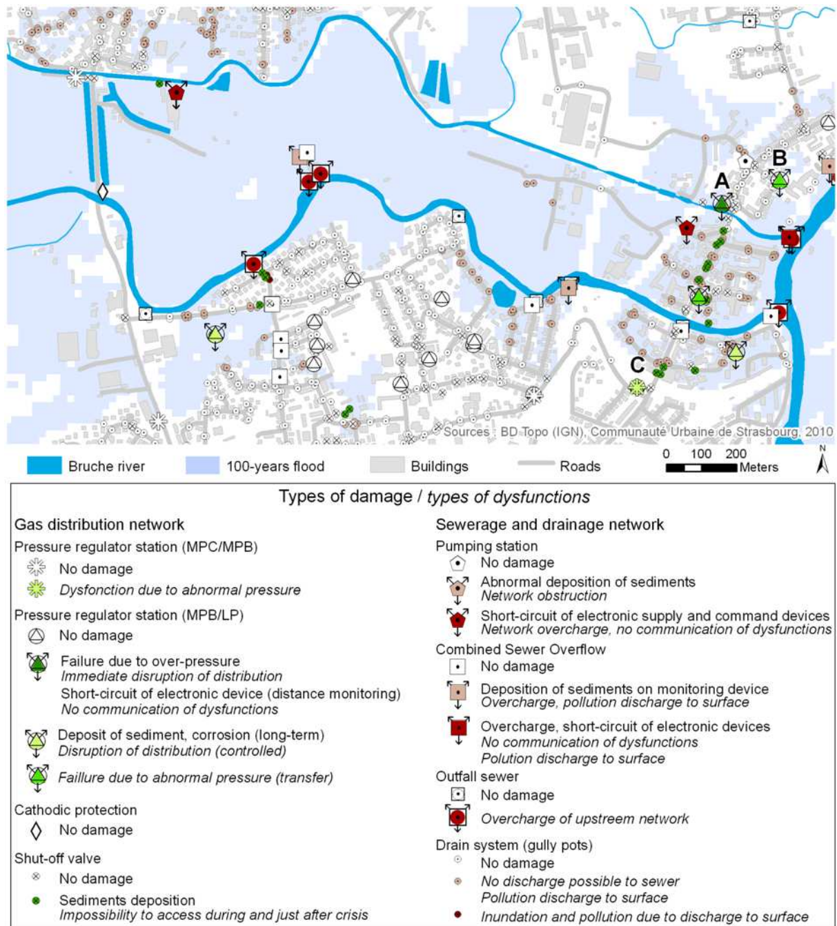
Figure 10.7. Map of damage-dysfunctions induced by a 100-years return-period flood for the components of gas distribution and sewerage/drainage networks.
