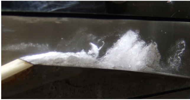
Fig. 21. Photograph of the cavity, 8° Venturi.
