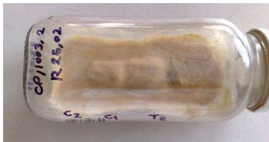
Figure 29- Agar-block test plates for WPC samples and control after 1 month.
