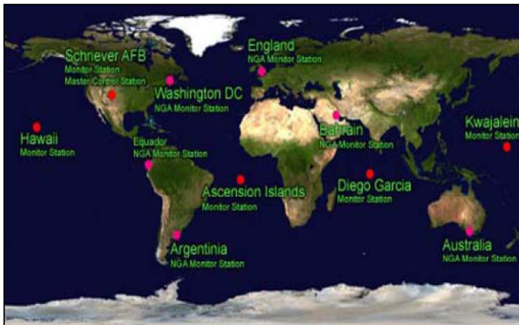
Figure 1.14: Global Positioning System (GPS) Master Control and Monitor Station Network [27, 78]
