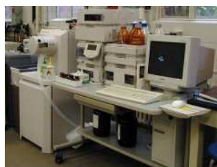
Fig. 19: LC-MS utilisé (Bruker Esquire Liquid Chromatograph - Ion Trap Mass Spectrometer)
