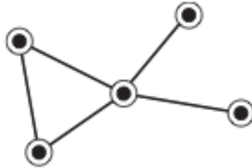
Fig. 2.2: Illustration of the definition of the clustering coefficient C . The individual vertices have local clustering coefficients, Eq. (2.5), of 1, 1, \frac{1}{6} , 0 and 0, for a mean value, Eq. (2.7), of C = \frac{13}{30} .
