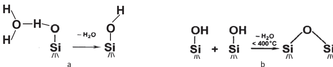
Scheme 1| a. Dehydration of physisorbed water on silica surface. b. Dehydroxylation reaction forming siloxane bridge by condensation.
