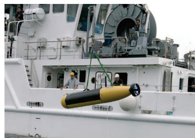
FIGURE 1.15 – AUV Muscle de Thales Underwater Systems et Bluefin Robotics [39]
