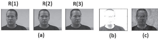
Fig. 2. Illustrating the saturation effect: (a) three 8 bit grayscale images. (b) Image obtained by a classical linear combination of the three images shown in (a). (c) Image obtained using an optimized merging (spectral segmentation).
