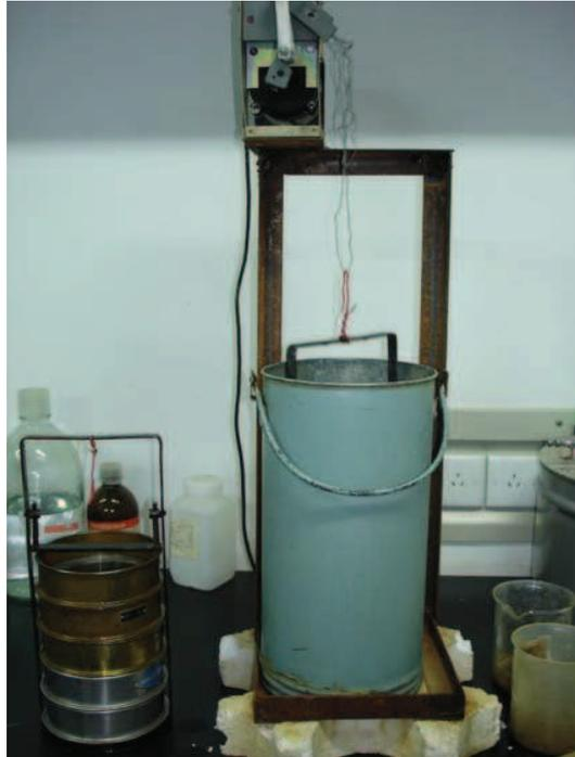
*Photo II.1: The Wet-sieving apparatus used in our experiment.*
