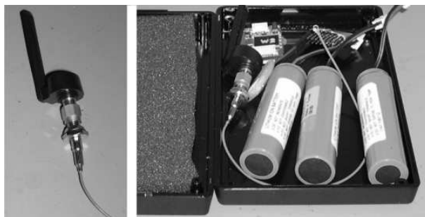
Figure 5.2: Long range iMote with rechargeable batteries.
