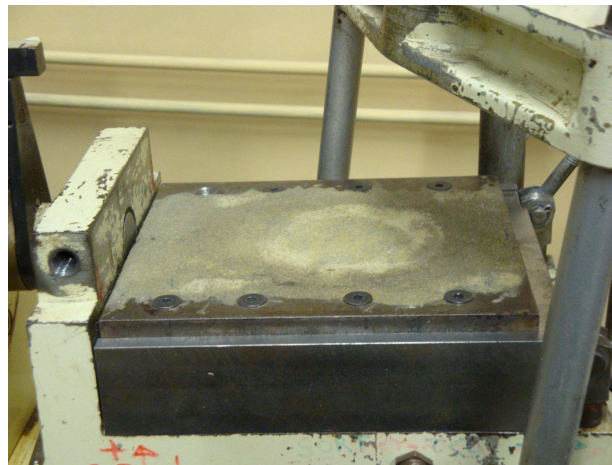
Figure 2.8: Rough surface positioned on direct shear test
