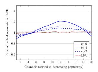
Figure 5.9: Stored segments for the channels of the time-shifted TV service.
