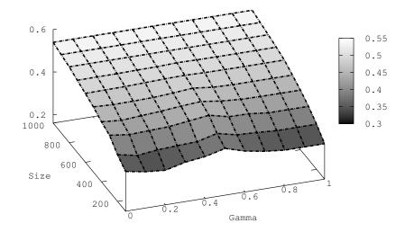
Figure 6.1: Single-cache simulation with static object popularity (On the y-axis, absolute hit-ratio produced by simulation.)
