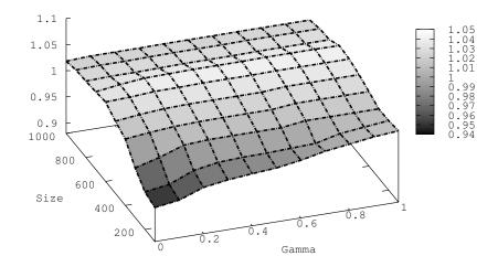
Figure 6.5: Comparison of approximation and simulation for a single cache with static object popularity (On the *y*-axis, ratio of hit-ratio approximation to hit-ratio simulation. The same in Fig. 6.6 and Fig. 6.11)
