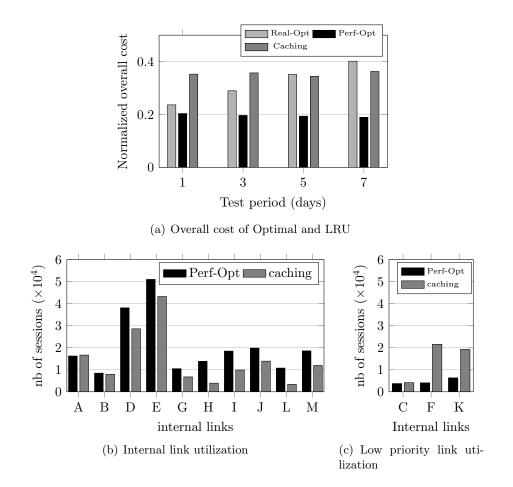
Figure 4.7: Optimal placement versus LRU Caching
