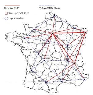
Figure 4.4: Envisioned telco-CDN topology in France. Three telco-CDN PoPs enable inter-connections with multiple traditional CDNs.
