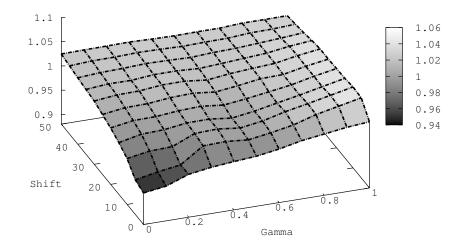
Figure 6.11: Comparison of approximation and simulation for a single cache with dynamic object popularity (On the y-axis, ratio of hit-ratio approximation to hit-ratio simulation).
