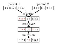
Figure 4.2: Creation of offspring: an example with three repositories, having respectively 3, 2 and 3 storage capacities
