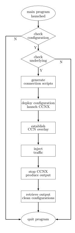
Figure 5.11: Execution Process of CCNxProSimu
