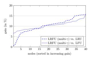
Figure 6.9: Gain in terms of hit ratio of LRFU (multi- $\gamma$ ) versus LRU and LFU
