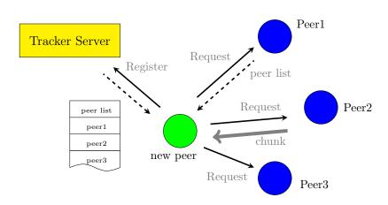
Figure 2.2: Bootstrapping in mesh-based P2P video streaming
