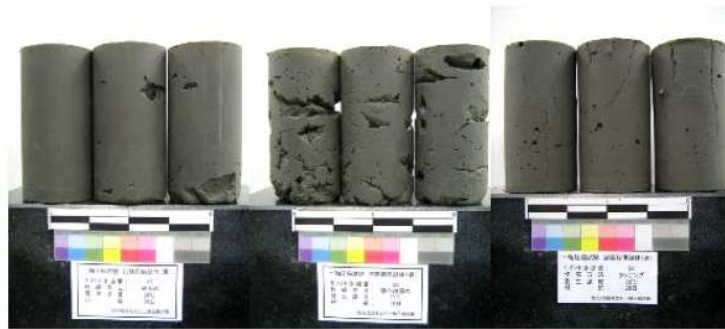
(a) Dynamic compaction (b) Static compaction (c) Tapping
