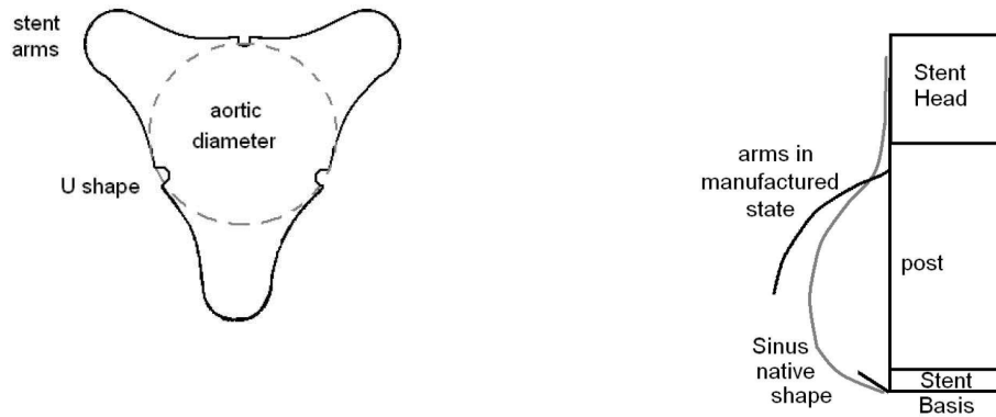
Fig III.8_Top and front representation of the stent arms
