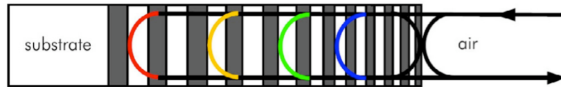
Figure 3.2.6. Structure of a chirped mirror operating based on the penetration effect. The mirror consists of multilayers that reflect wavelengths at different depths introducing group delay between the wavelengths. Diagram taken from [Rau 07].
