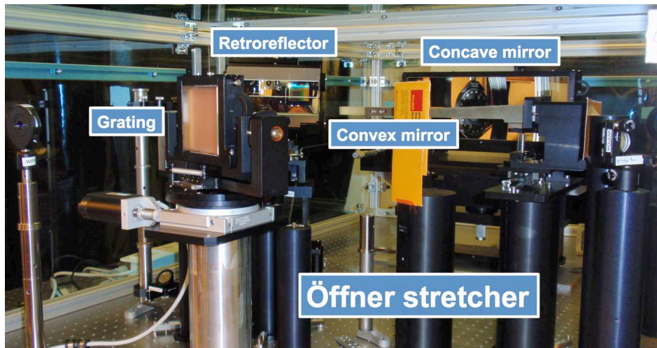
Figure 2.1.5. Öffner stretcher which will stretch the ps-pulses to 1 ns for the nanosecond OPCPA stage.
