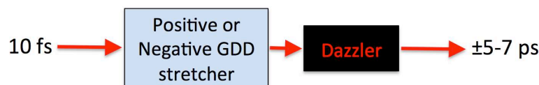
Figure 4.3.1. Block diagram representing the seed stretcher. Several elements to stretch the pulse positively or negatively are tested together with a Dazzler that will be used to correct higher order phase.
