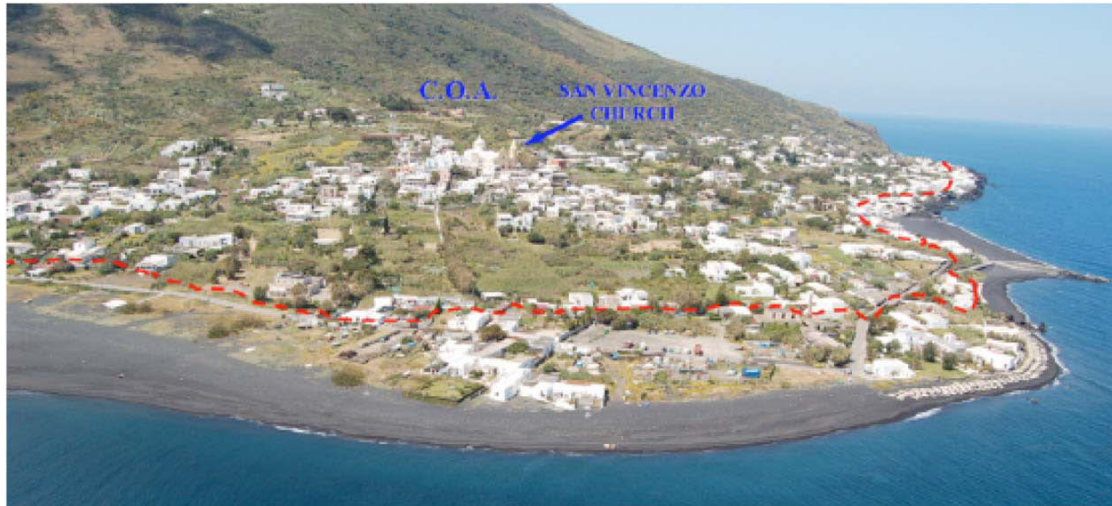
Figure 4: Northeastern coast of Stromboli island, showing the maximum run up of the December 2002 tsunami (red dashed line) and the operative center (COA) created by the Italian civil protection after the crisis of 2002-2003 (from Bertolaso et al., 2009).
