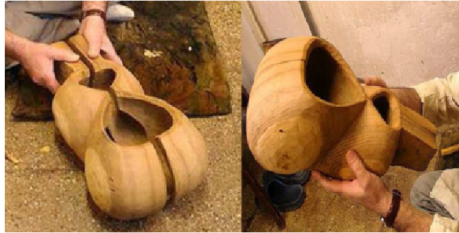
Fig.A.6. Attaching two completely carved halves together to form the final shape (Mr. Pouria's interview. Jadidonline magazine, 16 November 2007).
