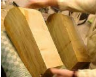
Fig.A.3. Two identical halves of white Mulberry's wood prepared for Târ fabrication (Yousef Pouria's interview. Jadidonline magazine, 16 November 2007).
