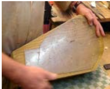
Fig.A.4. Fixing the pattern to the wood block (Mr. Pouria's interview. Jadidonline magazine, 16 November 2007).
