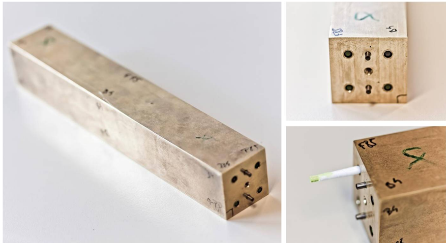
Figure 7.13: Pictures of the brass absorber containing the four LuAG fibers. This CFCAL was inserted among \text{PbWO}_4 crystals in the EE module facing the beam.
