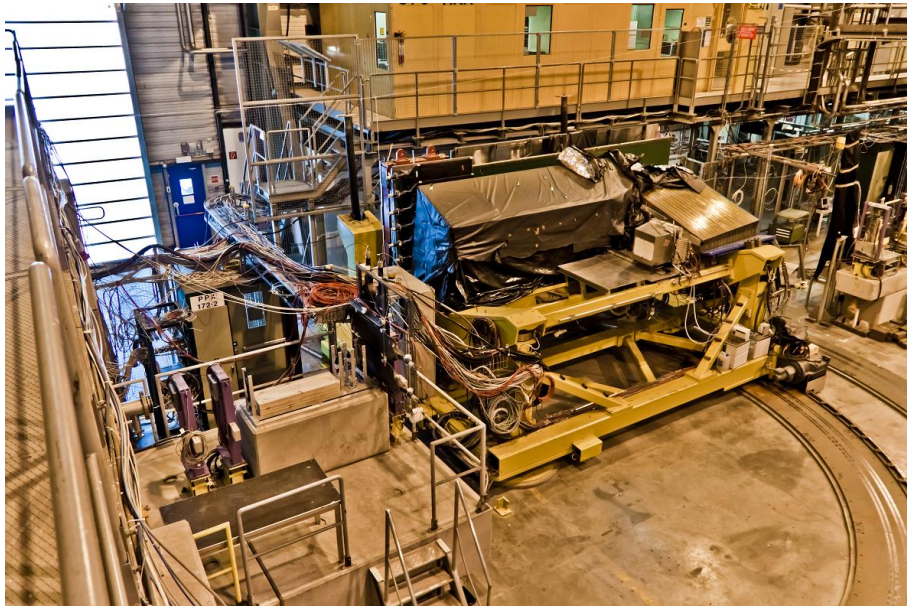
Figure 7.11: Picture of one of the experimental zones of H2. A wedge of the CMS detector (right side) faces the beam line and its triggering system (left side).
