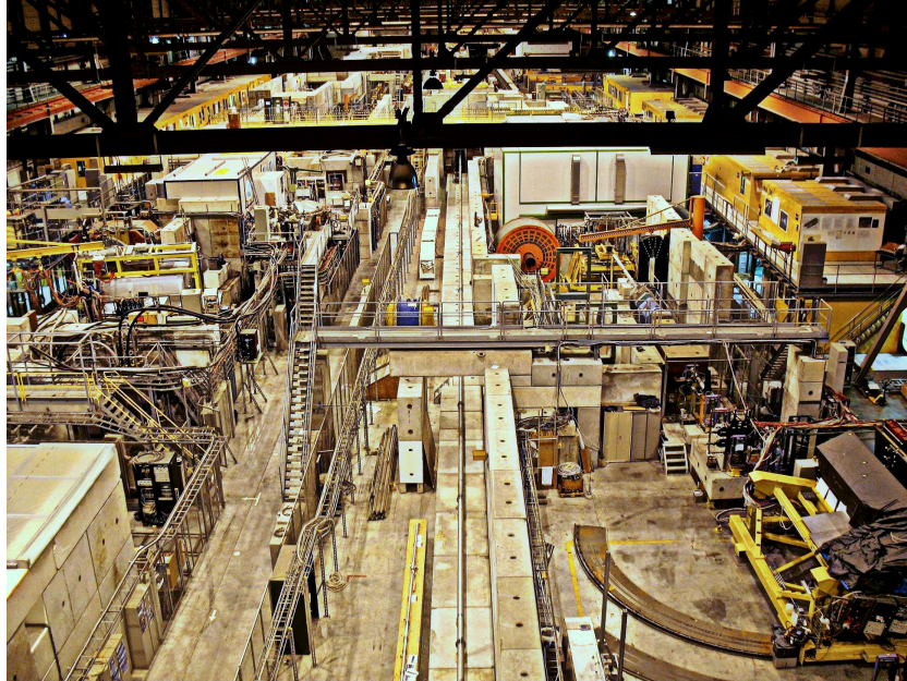
Figure 7.1: Picture of H2 (right side) and H4 (middle) beam lines at CERN. In front of H2, the movable stage holding a slice of the CMS detector is visible.
