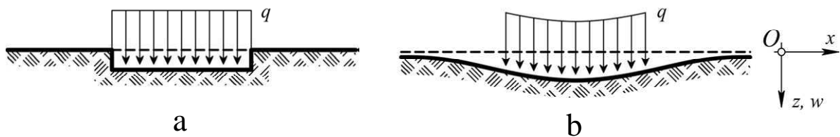
Figure 1-13: Deflections of elastic foundations under uniform pressure: a) Winkler foundation; b) Practical soil foundation.
