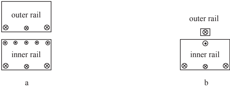
Fig. 6.5: Model for the current distribution for a large outer rail (a) and a small outer rail (b)
