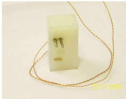
Fig. 4.17: Measurement device for the determination of the current distribution between the current brushes.
