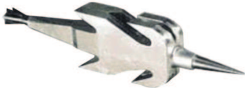
Fig. 1.13: C-shape solid armature with two current bridges [GAL04]
