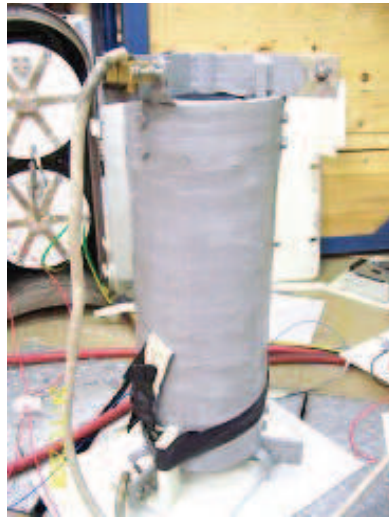
Fig. 4.5: Pulse forming coil ( L = 8 \mu\text{H} , R = 1.4 \text{ m}\Omega )
