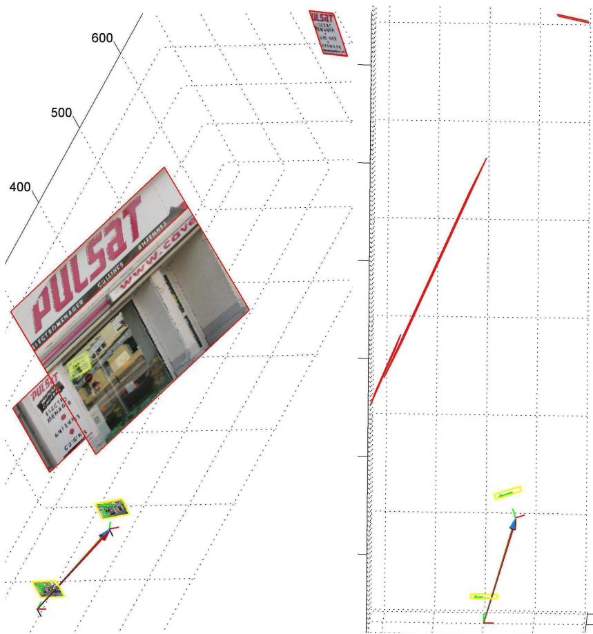
Figure 57: Reconstruction of 3 surfaces in the street view and estimated translation vectors in a unique frame.
