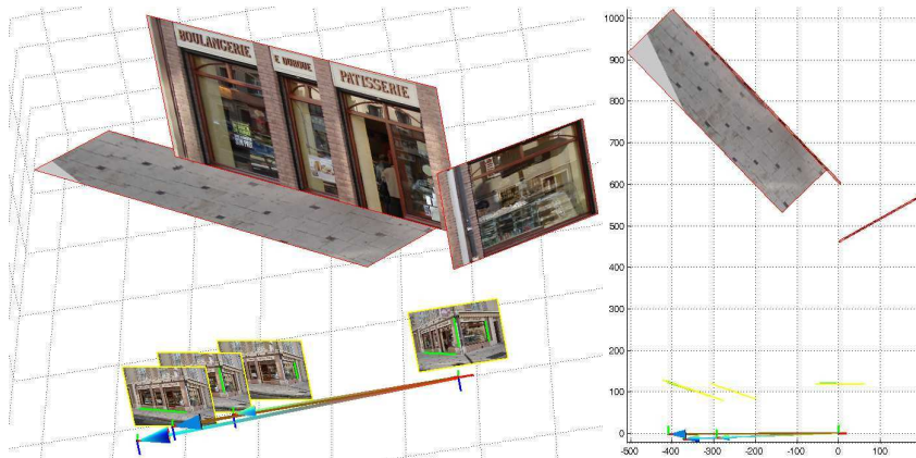
Figure 54: Reconstruction of the pavement and two walls of the bakery and 3 estimated translation vectors related to each surfaces. The scale of each surface reconstruction is different from others. The right image corresponds to the top view.
