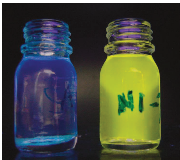
Figure 4.20. Picture of, left, a solution containing a mixture of concentrated NIOH ( 10^{-3} M) and diluted 3-(adamant-1-ylmethoxy)-6-chloro- s -tetrazine ( 5 \times 10^{-6} M) and, right, a diluted solution of NITZ ( 5 \times 10^{-6} M), under UV light irradiation (peak at 365nm).
