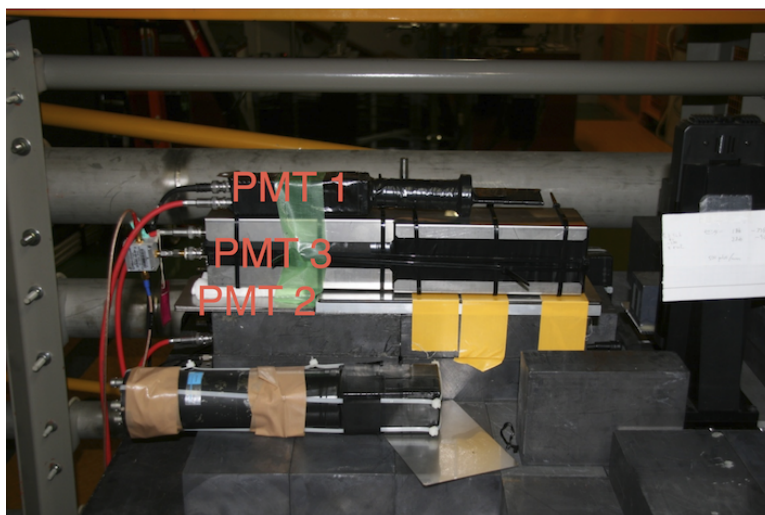
Figure 5.16: Schematic layout of the calibration setup - The two plastic scintillators read out by PMT 1 and PMT 2 are used to trigger the data acquisition of PMT 3 reading the \text{BaF}_2 crystal.
