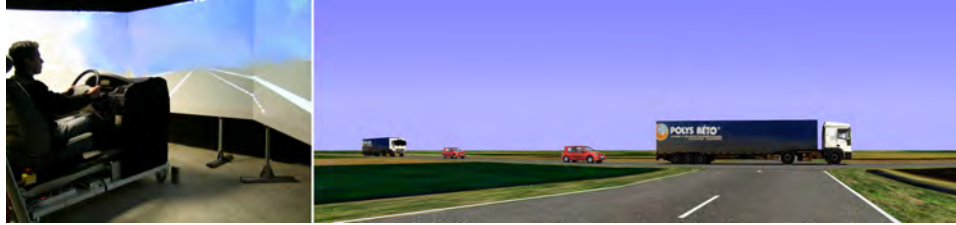
Figure 6.2.1: Simulator and simulated environment: controllers and screens (left panel); road crossing task with the two light vehicles defining the inter-vehicular Gap (right panel).
