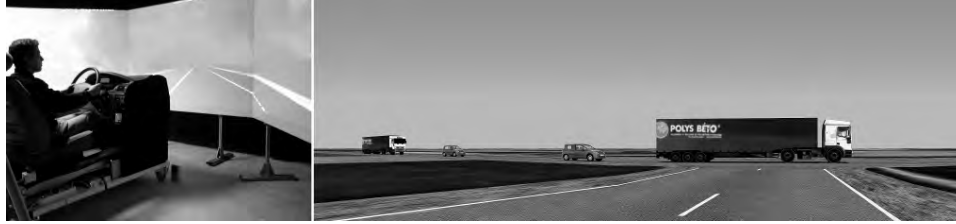
Figure 4.2.1: Illustration of the experimental setting (left panel) and the task's visual rendering as seen by participants (right panel). The task was to cross the intersection using the gap between the two cars.
