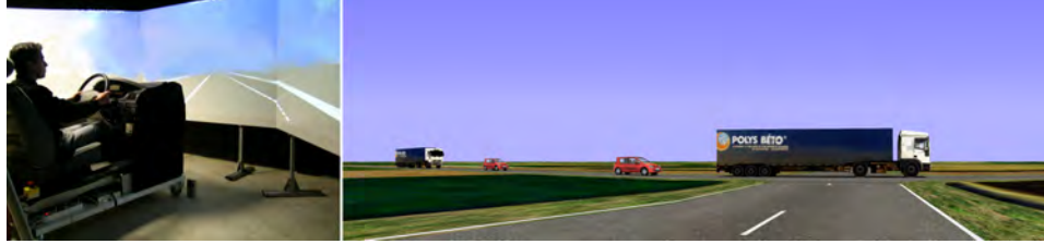
Figure 5.2.1: Illustration of the experimental setting (left panel) and the task's visual rendering as presented to the participants (right panel). The task was to cross the intersection using the gap between the two cars.
