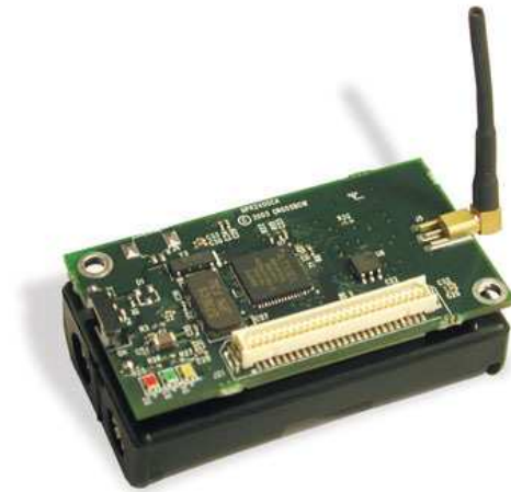
Figure 1.1: MICAz sensor mote hardware (Image courtesy of Crossbow Technology [xbow, 2004d])
