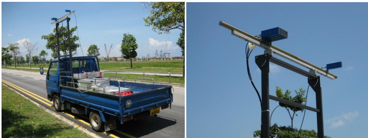
Fig. 5.4: Photographs of the ground-based passive radar test-bed on the moving lorry vehicle platform.
