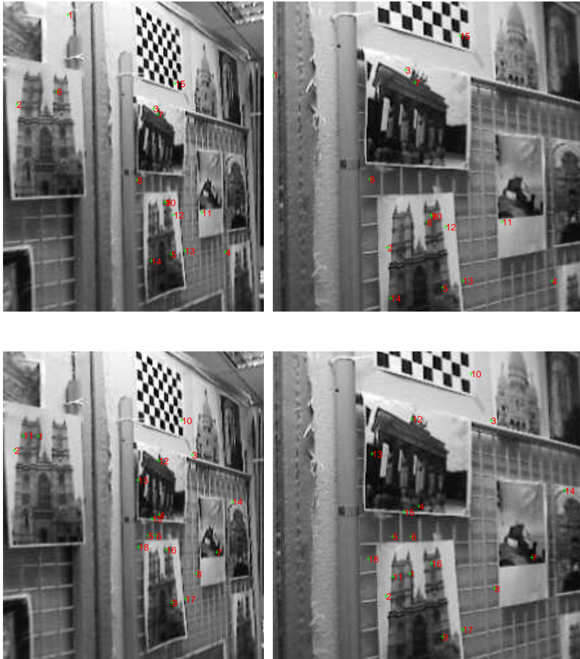
Figure 3.18: Comparing 2D-to-2D matches. Top row : Gaussian mean-shift G 80, Bottom row : Uniform mean shift U 175
