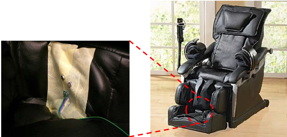
Figure 106 Illustration of sensor mounting on OSIM iDesire Massage Chair
