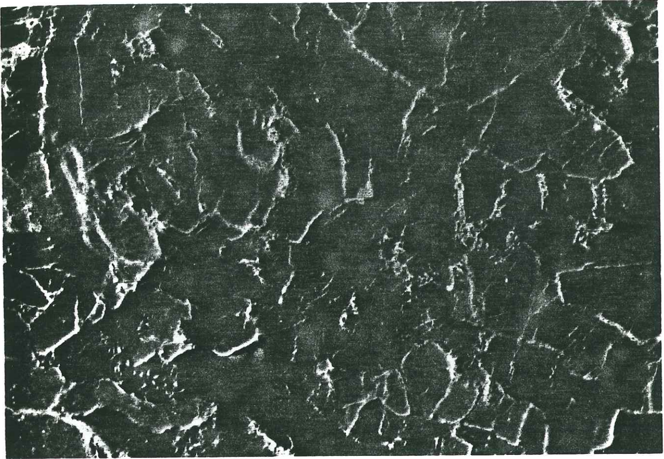
Fig. 7 This sample deformed in the transitional regime at 4 \times 10^{-5} \text{ s}^{-1} , under 300 MPa confining pressure, did not show any fault but did show a stable strain softening after reaching a peak stress of 470 MPa. Stress was applied vertically.
