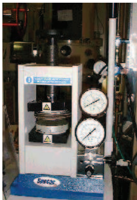
Figure 2.15 Hydraulic press with a pair of hot plates used in this work.
