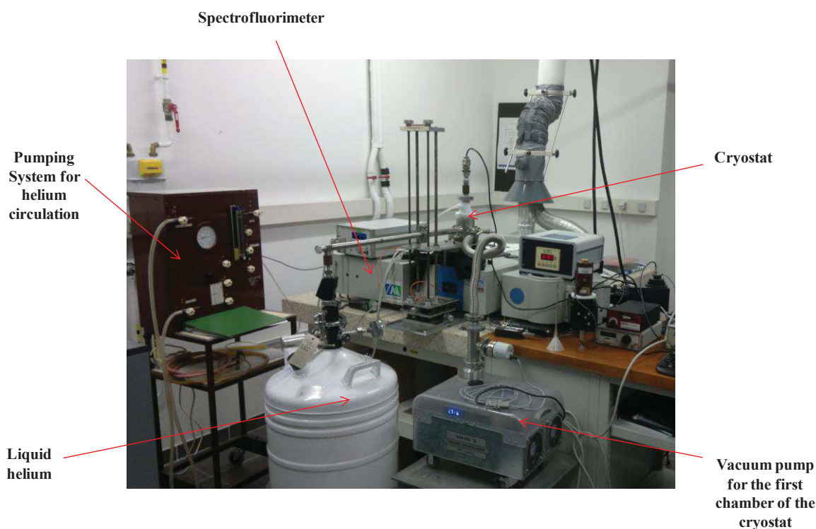
Figure A-2. Experimental set-up for fluorescence measurements at 4.2K (with liquid helium)
