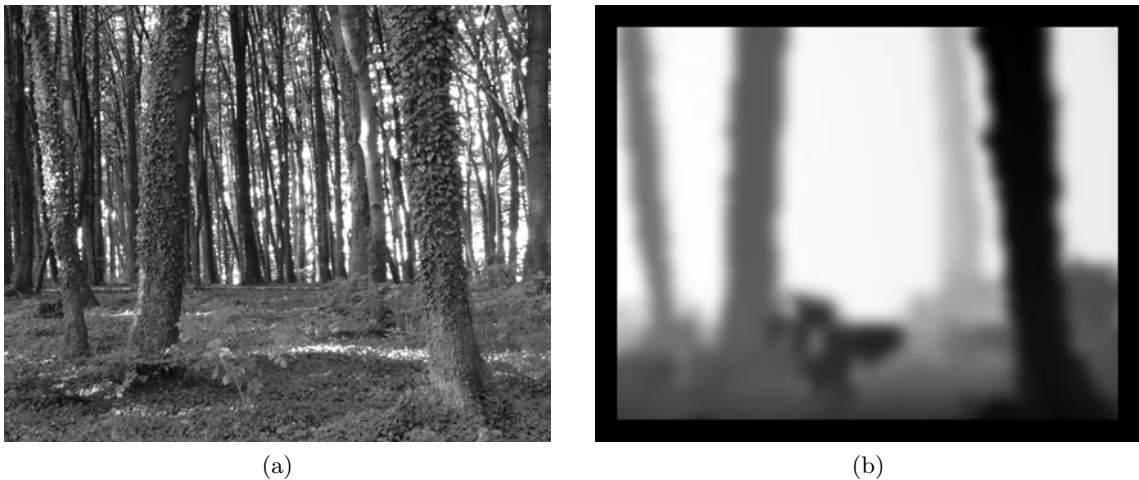
Figure 2.4: Original picture (left) and its disparity map (right) (black areas stand for the closest areas whereas the bright areas indicate the farthest ones).
