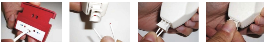
Figure 1.6: Firecomms point-to-point link at 100Mbit/s with its Do It Yourself kit, from [3].
